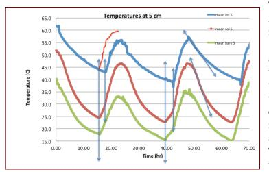
This graph is very illustrative. At 5 cm. depth, the temperature maxima of the soil in the 'insulated' beds (blue curves) are 10 C higher than those in the solarized beds (tan curves), which are 15 C higher than those in bare ground (green curves). The temperature minima for the three treatments are 40, 23, and 15, respectively. The rate of cooling (slope of the lines) is much higher in the
