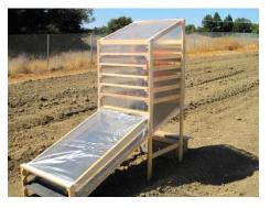
into the cabinet dryer. Samples of fruit were placed on small sections of plastic mesh and were weighed approximately every two hours to monitor tomato moisture content. Inlet air and exhaust air temperatures were recorded for both dryers.
