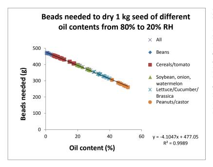
Figure 1. Amounts of drying beads needed to dry 1 kg of seeds of different oil content from equilibrium with 80% to 20% RH. As the seed oil content increases, the amount of beads required decreases linearly. This relationship is used in the Bead Calculator to determine the amount of beads needed to dry seeds of a specific species from an initial RH (MC) to a final RH (MC).
