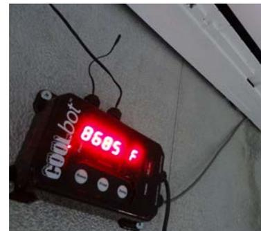
Above, a CoolBot connects to an air conditioner to further lower the thermostat without freezing over so that a well-insulated room can cool fresh produce effectively.
