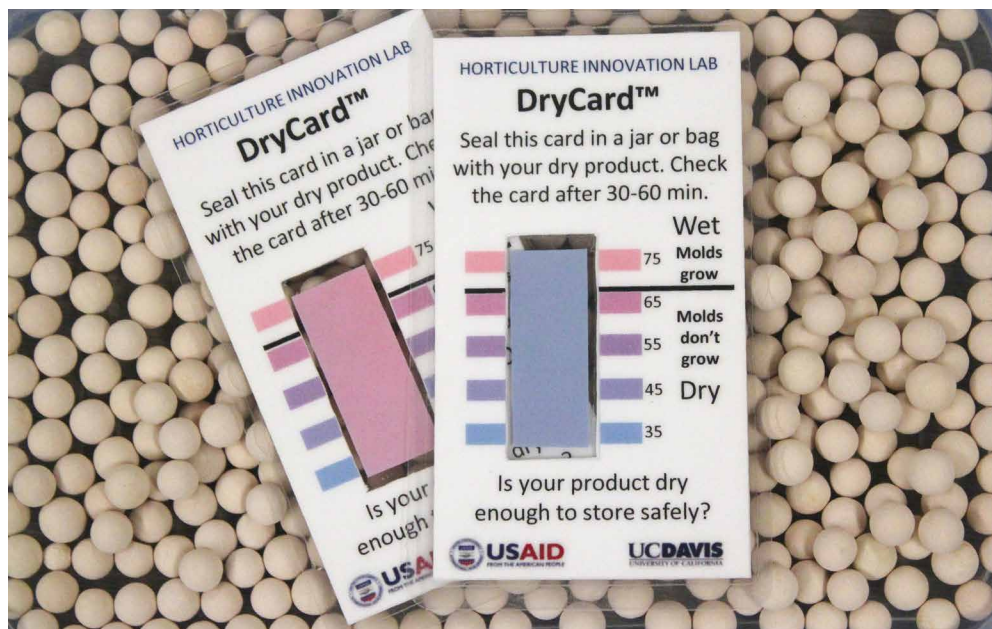
By combining a strip of cobalt chloride paper with a color index, the DryCard indicates by color whether dried foods are dry enough to store safely, reducing the risk of mold growth. (Horticulture Innovation Lab photo by Brenda Dawson/UC Davis)
