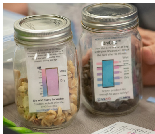
DryCard™ dryness indicator. Pink is not sufficiently dry, purple or blue is sufficiently dry.
