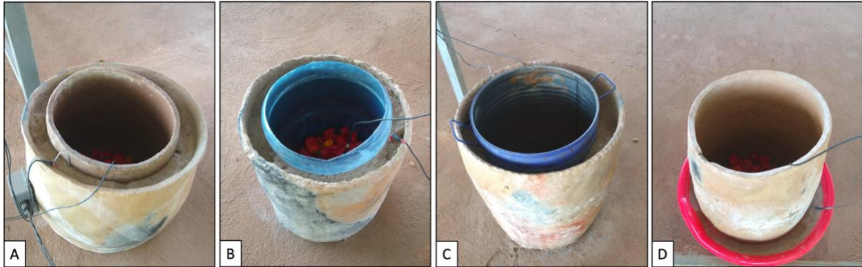
Figure 12. Examples of the 4 clay pot cooler designs studied at each of the three locations in Rwanda.
