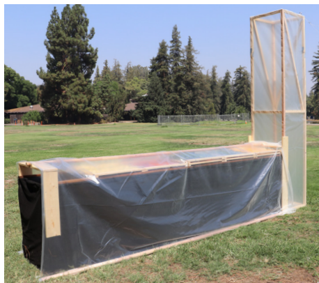
Four main components to the chimney solar dryer, clockwise from top left: a drying table, a chimney, mesh trays, and clear film to cover the drying table.
