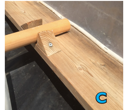
Left and top right: An additional pole support in the center of the table to reduce sagging. Bottom right: small blocks of wood on the center pole support shelves prevents pole from rolling.
