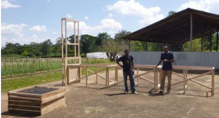
Wood Frame and 1m 2 trays for UCD chimney dryer. This shows the plywood between the table and chimney, which we got from the original Uzbekistan photo that MS Reid gave to the PI during proposal development. We decided after prototyping in TZ that it was expensive and not needed.
