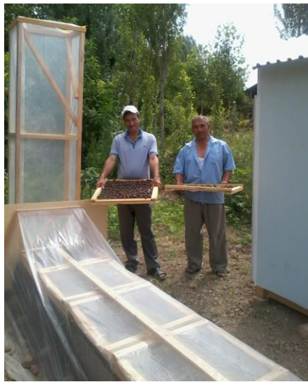
UCD solar chimney dryer with 2 meter tall stack chimney (left) and the traditional Indirect Solar Cabinet Dryer with Solar Collector, 4 Drying Trays and small metal chimney with umbrella cap (right)
