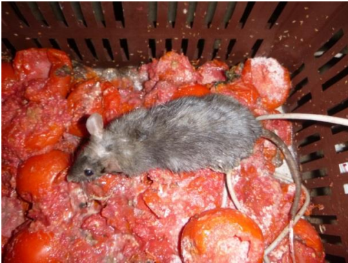
Rat in ZECC experimental plastic crate in Tamale, Ghana (Trial #1 -- the subsequent trial incorporated a rat proof wire screen mesh)
