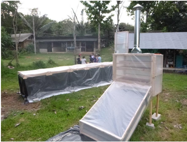
Indirect solar cabinet dryer constructed in Chiang Mai, Thailand showing chimney with a “Chinese cap” style cover.
