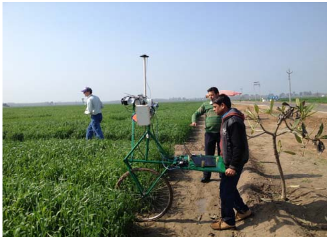
Phenocart with sensors and GPS used in field measurements
