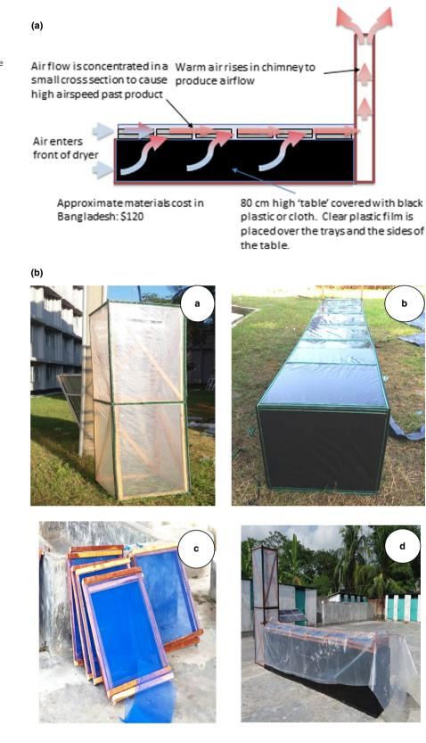
using a digital thermometer (AMF026, Qingdao, Shandong province, China). Fish was dried daily from 9 a.m. to 5 p.m. Temperature monitoring was conducted at 10 a.m., 1 p.m., and 4 p.m. both inside and outside of UC Davis solar chimney dryer. The results of the temperature reading are shown in Table 1.
